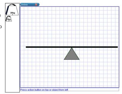
To earn two points, a student must place the 5 kg weight four times as far from the fulcrum as the 20 kg weight, as shown in the example below.
